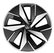
STANDARD ON ID.4 GTX 20" 'Ystad' alloy wheels 8J x 20 in front, 9J x 20 in rear Tyres: 235/50 R20 in front 255/45 R20 in rear
